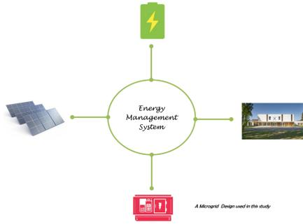
The study goal is to create a **smart EMS** to manage the power dispatch of a microgrid to minimize the operation costs, while maintaining the grid stability: the **Economic Dispatch** is an optimisation problem
